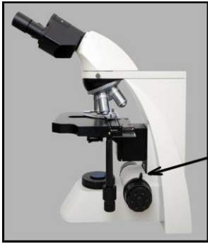
Examples of an Auto-Stop Mechanism that prevents objectives from hitting the slide
